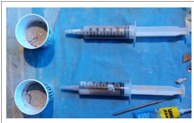
Figure 17. Injectors and cups used to monitor the bleeding water, shrinkage amount, and setting status of the trial grouts prepared at the worksite for injection.
