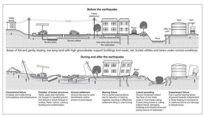
Figure 12. Soil liquefaction and its impact on underground structures (Mian et al., 2013).
