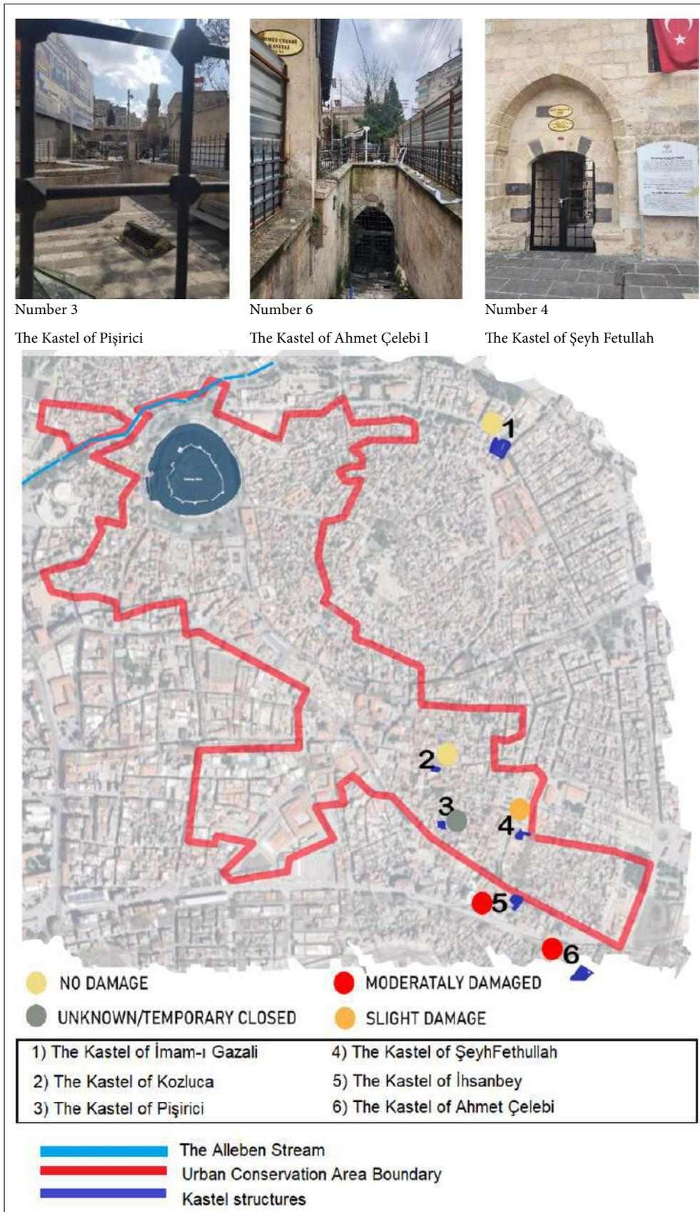
**Figure 5.** According to reports, the post-earthquake situation of the Kastels in Gaziantep City Center.
