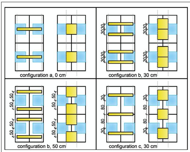
**Figure 8.** Luminaire configuration examples for quadruple desk layout.
