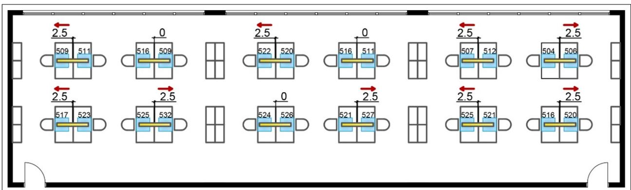
**Figure 9.** Example of shifting luminaires in the direction of the line of sight and vice-versa in a dual desk layout: RD-3, configuration a, 0 cm.
