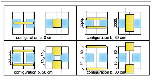
**Figure 7.** Luminaire configuration examples for dual desk layout.
