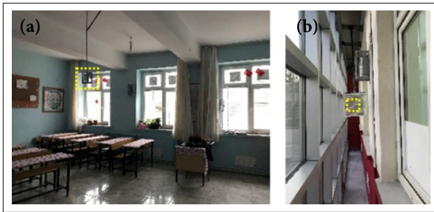
Figure 7. Ambient temperature measurement device locations (a) Test classroom (b) Cavity.
